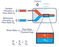
Images acquired during the measurement allow the software to calculate the position of the interface and directly plot an interactive flow curve.
